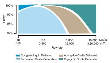
PSA can produce nitrogen in a range of purities as shown in figure 1. However, figure 1 does not take into account the financial aspect (i.e. the cost of production). Figure 2 can give an idea of the general trend of how costs change with increasing levels of purity and increasing flow rates. It is not always necessary to produce highly pure nitrogen. For example, blanketing vegetable oils can be done with purities of around 99.5%.
