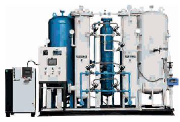
Pressure Swing Adsorption (PSA) is a nitrogen gas generation method with a specially designed adsorbent. This adsorbent is called a Carbon Molecular Sieve (CMS) having micro pores in its surface to adsorb O2, CO2, and H2O molecules when under a certain pressure. After the adsorption process, the adsorbent is regenerated by
